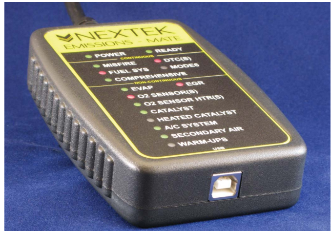
Emissions-Mate HandHeld Unit shows USB 2.0 Full Speed Type-B Connector
